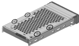
Figure 2-4-2. Installing 3.5-inch SAS/SATA Drive
