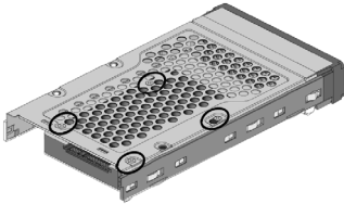
Figure 2-4-1. Installing 2.5-inch SAS/SATA Drive
