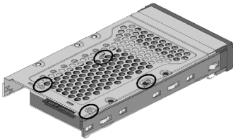
Figure 1-4-1. Installing 2.5-inch SAS/SATA Drive
