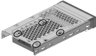
Figure 2-4-1, Installing 2.5-inch SATA Drive
