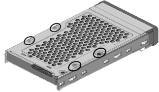
Figure 2-4-2, Installing 3.5-inch SATA Drive
