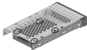
Figure 2-7. 2.5-inch Drive Carrier with 3.5-inch SAS/SATA Drive
