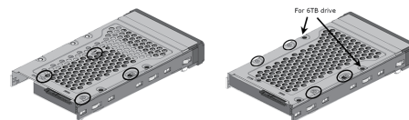
Figure 4, Secure the 2.5/3.5-inch Drive to the Tray
