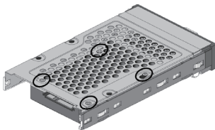
Figure 2-4, Drive carrier with 2.5-inch SAS/SATA drive
